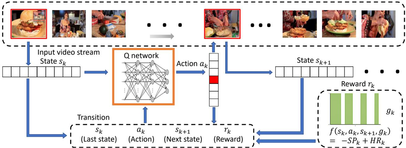
Figure 2. **Model of our FFNet.** We learn a strategy for fast-forwarding videos. At each time step  $k$  we use the Q network to select the action  $a_k$ , i.e., the number of frames to skip next. The state  $s_{k+1}$  is updated with the frame it jumps to. Then, the reward  $r_k$  for action  $a_k$  in state  $s_k$  is computed with the interval annotation  $g_k$ . A transition in a quadruple form  $(s_k, a_k, s_{k+1}, r_k)$  is used to update the Q network.
