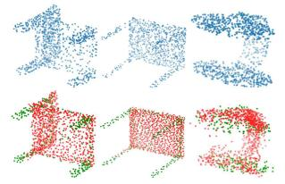
Figure 5. Examples of point cloud autoencoder results. First row: input point clouds of size 1024. Second row: reconstructed point clouds of size 1280. From left to right: chair, table, earphone.
