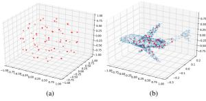
Figure 2. (a) The initial nodes of an  $8 \times 8$  SOM. For each SOM configuration, the initial nodes are fixed for every point cloud. (b) Example of a SOM training result.
