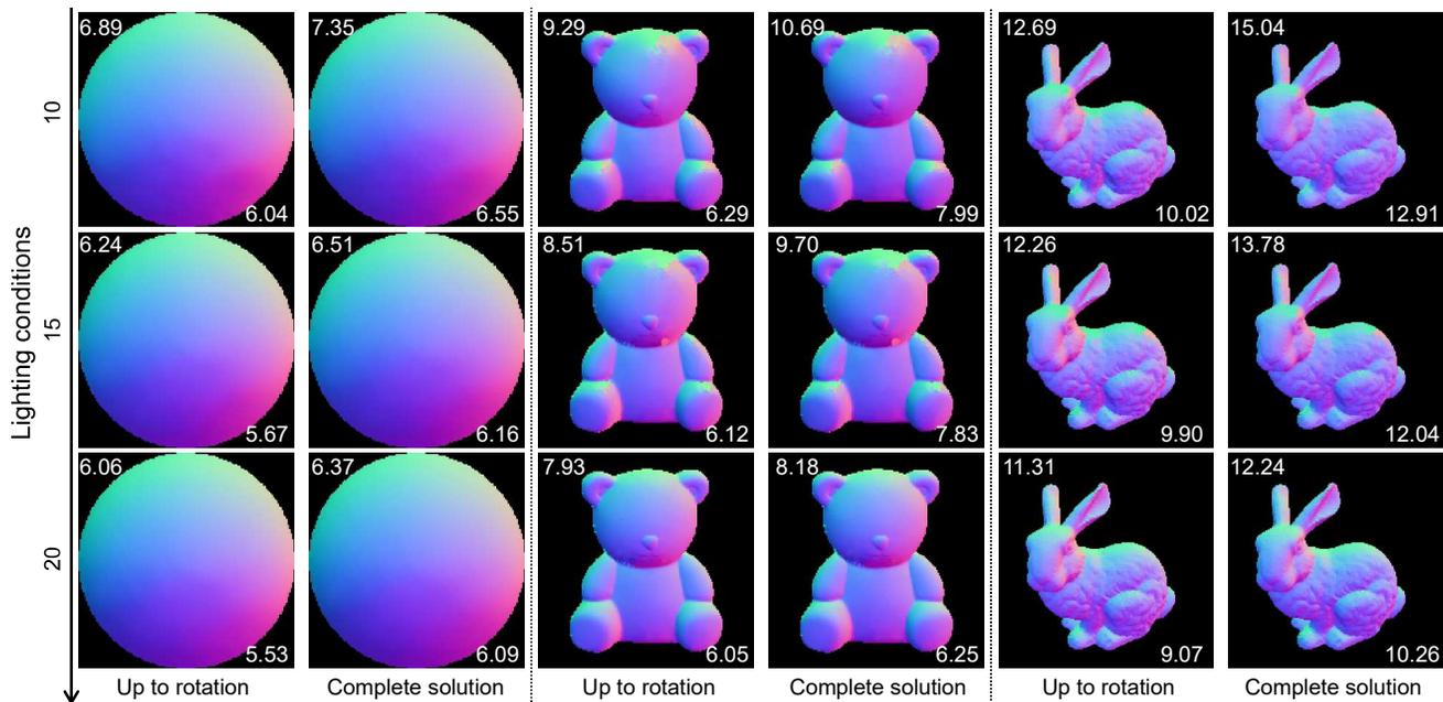
Figure 6. Normal estimation results varying with lighting conditions. We show the estimated normal maps using different numbers of input images (10, 15, and 20). The numbers on the upper left and bottom right corners of the normal maps show the mean and median angular errors w.r.t. to the ground truth (shown in Fig. 5). For each data, we show results up to rotation in which we use ground truth to resolve the global ambiguity and the results from our complete solution.
