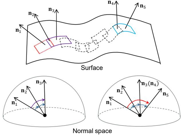
Figure 4. Angular distance propagation through shortest path.
