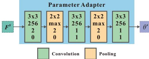
Figure 3. The architecture of the parameter adapter in PIL. The parameter adapter takes the features  $F^S$  from the parsing encoder as input and outputs the adaptive convolution parameters  $\theta'$ . It is composed by stacking three convolution layers and two pooling layers. For each layer, the kernel size, the number of channels/pooling type, stride and padding size are specified from top to bottom.
