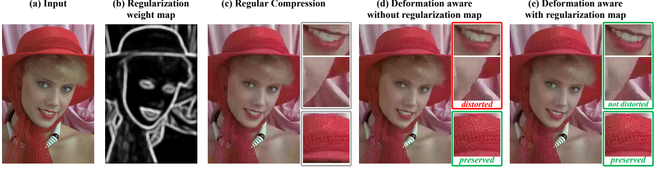
Figure 8. The effect of the regularization weight map. Applying our scheme (with WebP compression at a ratio of 250:1) on image (a) without adaptive regularization (constant w(\xi, \eta) ), results in image (d) in which the hat’s texture is better preserved, compared to the regular WebP compression (c), but the woman’s lips are distorted unrealistically. Using the local regularization weight map (b), results in image (e) in which the boundaries of the lips are not distorted, yet the texture on the hat is still sharper than with the regular compression (c).
