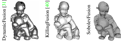
Figure 7. Canonical model comparison on the full-loop Squeeze sequence from DynamicFusion [31]. SobolevFusion recovers the fine structures on the face better than KillingFusion [40].
