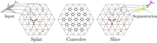
Figure 2: **Bilateral Convolution Layer.** *Splat*: BCL first interpolates input features  $F$  onto a  $d_l$ -dimensional permutohedral lattice defined by the lattice features  $L$  at input points. *Convolve*: BCL then does  $d_l$ -dimensional convolution over this sparsely populated lattice. *Slice*: The filtered signal is then interpolated back onto the input signal. For illustration, input and output are shown as point cloud and the corresponding segmentation labels.
