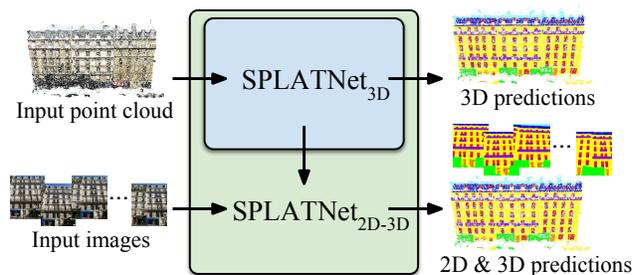
Figure 1: **From point clouds and images to semantics.** SPLATNet<sub>3D</sub> directly takes point cloud as input and predicts labels for each point. SPLATNet<sub>2D-3D</sub>, on the other hand, jointly processes both point cloud and the corresponding multi-view images for better 2D and 3D predictions.
