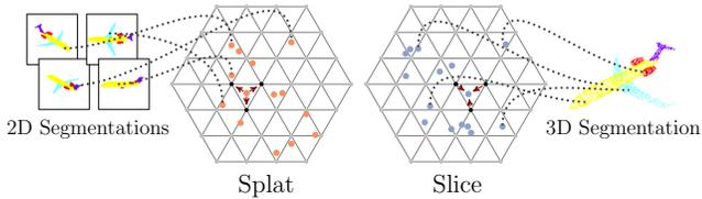
Figure 5: **2D to 3D projection.** Illustration of 2D to 3D projection using *splat* and *slice* using *splat* and *slice* operations. Given input features of 2D images, pixels are projected onto a 3D permutohedral lattice defined by 3D positional lattice features. The splatted signal is then sliced onto the points of interest in a 3D point cloud.
