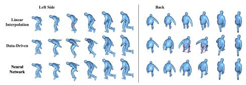
Figure 4. Comparison of mesh interpolation results. First row is the result of direct linear interpolation of the RIMD feature, second row is the result of [8], third row is our result. All the results are shown in two views, with artifacts marked using red circles.
