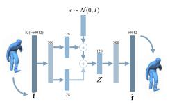
Figure 1. Pipeline of mesh VAE. The model in the figure has 2502 vertices and 7500 edges. Each dR of a directed edge has 3 elements, and  ${\bf S}$  of each vertex has 6 elements, so the total feature dimension  $K=2502\times 6+7500\times 3\times 2=60012$ .
