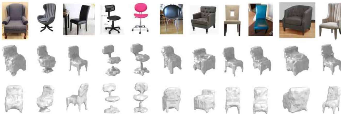
Figure 7: Visualization of predictions using the Stanford Online Product Dataset. (Top) Input image. (Middle) Predicted shape in the emergent canonical pose. (Bottom) Predicted shape rotated according to the predicted pose.
