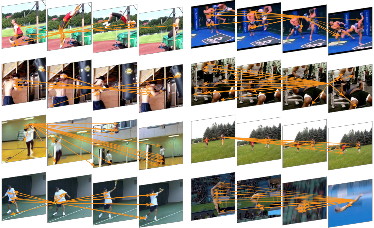
Figure 3. Examples of the behavior of a non-local block in \text{res}_3 computed by a 5-block non-local model trained on Kinetics. These examples are from held-out validation videos. The starting point of arrows represents one \mathbf{x}_i , and the ending points represent \mathbf{x}_j . The 20 highest weighted arrows for each \mathbf{x}_i are visualized. The 4 frames are from a 32-frame input, shown with a stride of 8 frames. These visualizations show how the model finds related clues to support its prediction.
