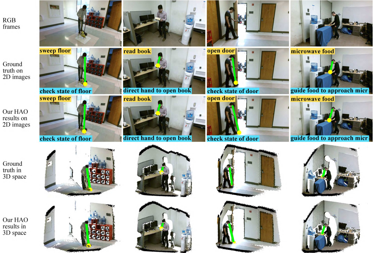
Figure 7: Visualization of intention prediction, attention prediction, and task recognition results. The texts on the RGB frames are the task label and intention label, respectively.
