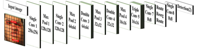
Figure 4. The proposed Palsynet consists of 4 blocks with 11 convolution layers and 4 max-pooling layers. The last Route-Reorganization-Route and a convolution layer are for multi-block feature extraction.
