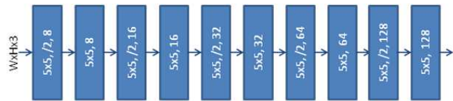
Figure 3. Baseline network with convolution blocks (/2 indicates downsampling, the last number indicates number of channels)
