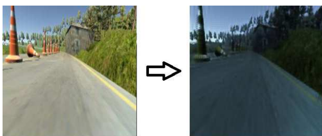
Figure 9. Using conditional GANs for data augmentation of one-shot corner case recording into other modes
