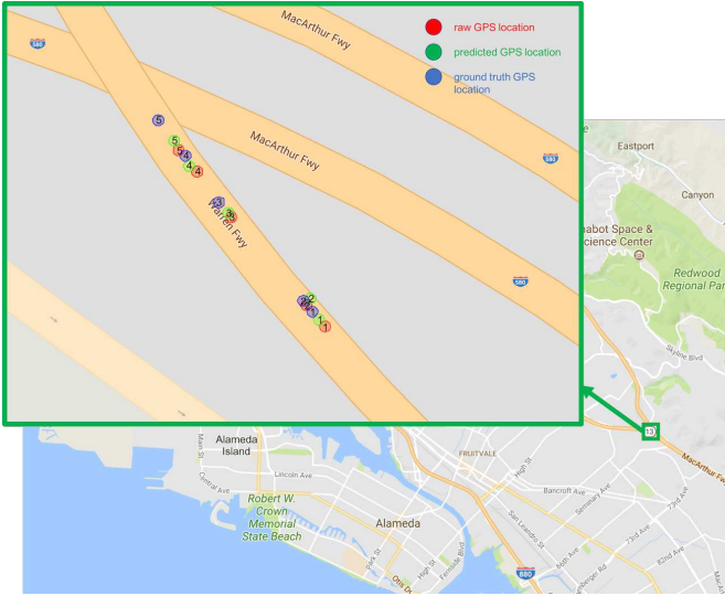
Figure 4: Five randomly picked points shown on the real map. Raw points colored in red. Predicted points are colored in green. True points are colored in blue.
