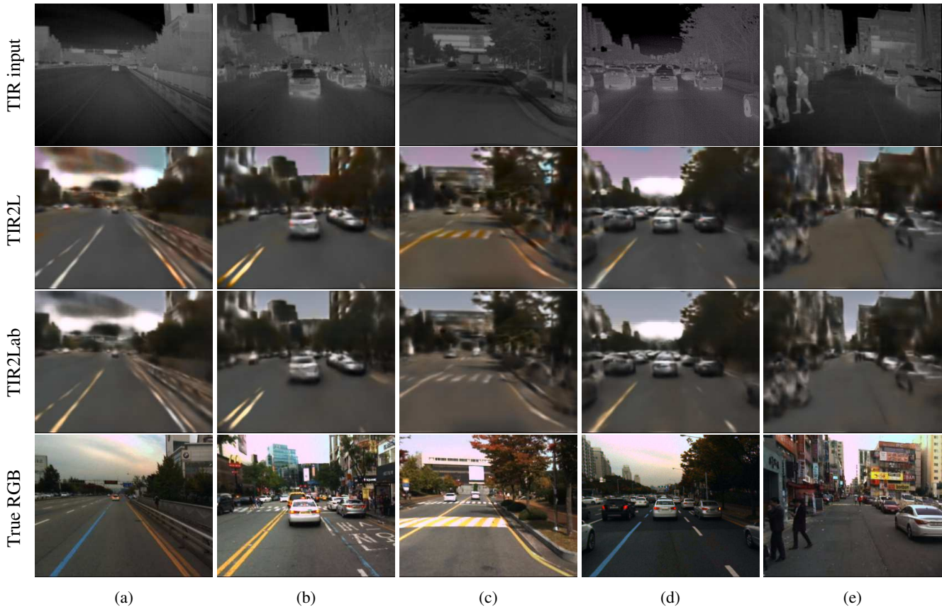
Figure 5: Failure cases for the proposed methods, first row shows input TIR image, second row the output from TIR2L, third row the output from TIR2Lab, and fourth row the true RGB images.
