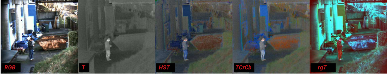
Figure 4. Exemplar RGB, infrared and varying visible-infrared fusion models (left to right).
