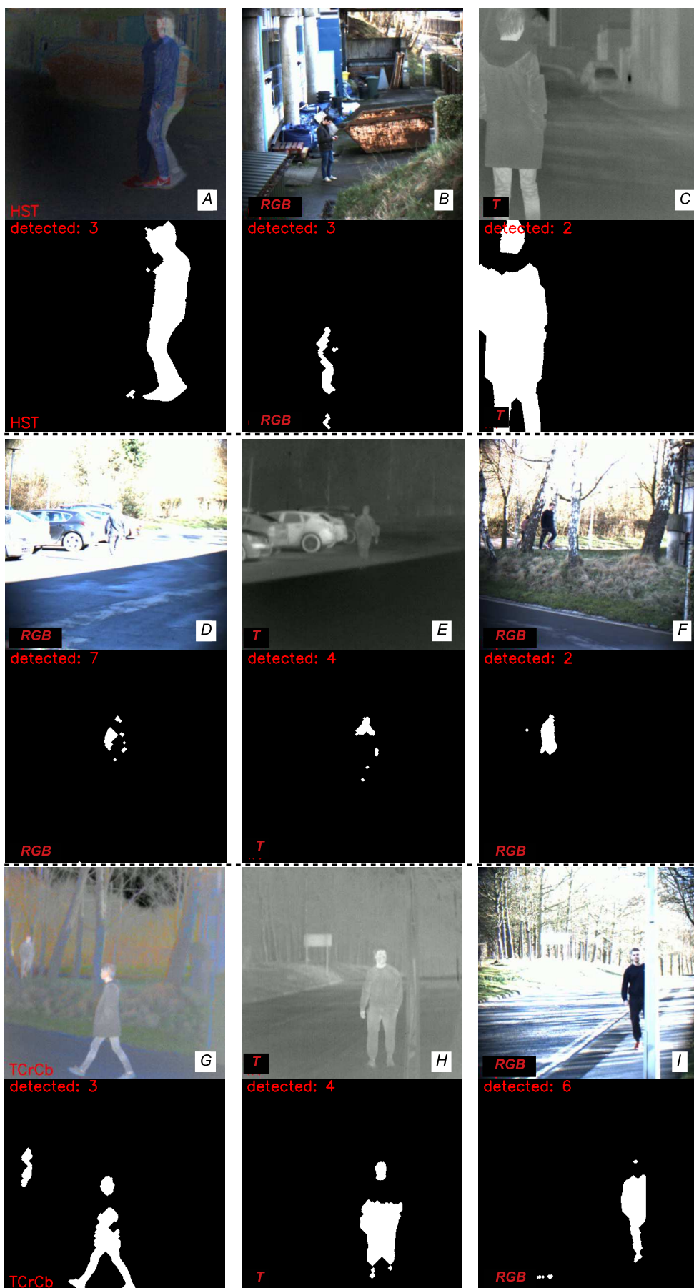
Figure 7. Exemplar foreground object detection - failure cases (A - I).
