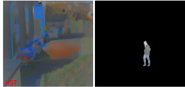
Figure 1. Exemplar - a background model (left) and extracted foreground object (right) using the HST fusion model.
