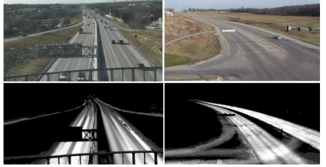
Figure 4. Estimated traffic flow density on two video sequences: (Top) original frames. (Bottom) motion flow densities.
