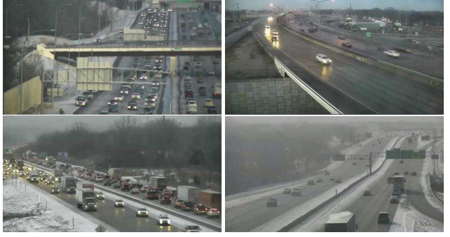
Figure 3. AIC18 Track 2 videos provide real-world challenges for anomaly detection: glare, occlusions, day/night views, high traffic volume, low contrast, camera vibration and compression artifacts.
