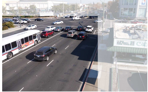
Figure 4. Example of considered ROI for location 4 of NVIDIA AI city challenge. It can be appreciated how the farthest vehicles are ignored, thus trading off the detector recall for an improved precision. Detections which are ignored are the most difficult and it would be very hard to track them successfully. Since in the successive phase tracklets are used to label the challenge videos we choose to privilege the precision w.r.t. the recall of the tracker.
