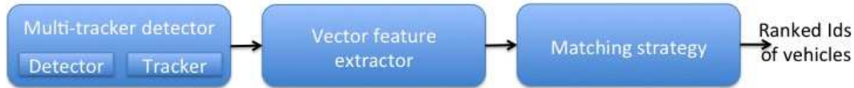
Figure 2. Our system pipeline that is composed of three modules. The first phase is vehicle detection and tracking. Detections are either assigned to an existing tracklet or used to initialize a new tracker. Tracklets are exploited to automatically annotate the videos and train a triplet network for vehicle re-identification. The output vector of the triplet network is used as feature vector to represent each detected vehicle. Eventually, these feature vectors are compared between different probes and the gallery to generate a ranking. We refer the reader to Section 3 for further details.
