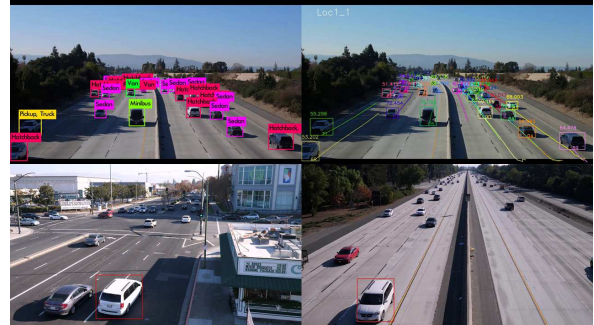
Fig. 1. Object detection, SCT with 3D speed estimation and multi-camera tracking. The detected vehicles and their car types are shown on top left . The trajectories of objects are shown on top right with the estimated speed in mi/h plotted above each bounding box. At the bottom , a pair of identified vehicles in two camera views are shown in red bounding boxes .
