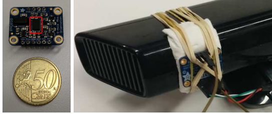
Figure 3. BNO055 board on a Kinect V1 RGB-D Camera.
