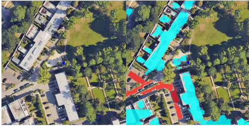
Figure 5: Buildings segmented using U-Net (Left: an EO image. Right: EO image overlaid with segmentation results).
