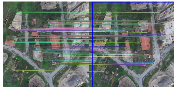
Figure 4: Registration of S_{(i)} and S_{(i+1)} using matched ORB features.
