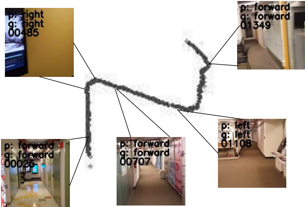
Figure 7: Example visual path captured using a smartphone (Samsung Galaxy Edge S6+) with 46 degree vertical FOV. Two image sequences were captured, one for training and the validation shown above using the same procedure as described in the experiments.
