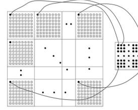
Figure 2. Subsampling procedure for DCTR feature extraction.
