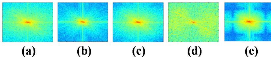
Figure 3. Power spectral density of the *Lena* image: (a) Original (Unfiltered); (b) Median filtered; (c) Gaussian filtered; (d) Laplacian filtered, and, (e) Average filtered.
