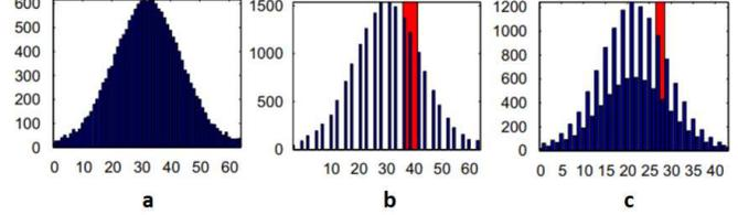
Figure 4. Example histogram of DCT coefficients in (a) single-compressed JPEG image; (b) and (c) double-compressed JPEG image. The case shown in (b) with periodically missing values happens when the first compression quality factor is not less than the second quality factor, and case (c) with periodic peaks and valleys happens when the first compression quality factor is less than the second quality factor. The shaded rectangles represent one period of the histograms.
