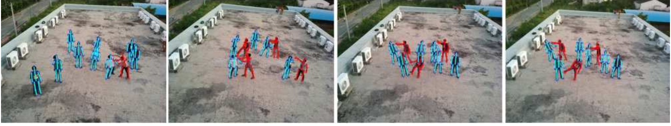
Figure 7. The figure shows the performance of the Drone Surveillance System (DSS) on aerial images with multiple humans engaging together in different violent activities. The violent individuals are highlighted in red color and neutral human in cyan color.
