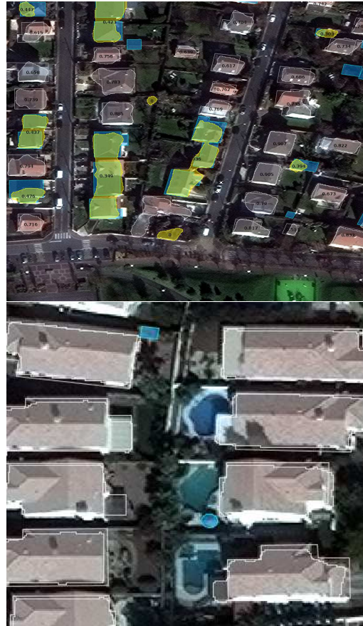
Figure 1. Example of errors. In the first image adjacent buildings are fused because they were too close from each other. In the second image only the big buildings have been detected while the little roofs have not.
