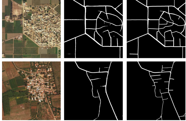
Figure 4: Example results of our road extraction method with an IoU score of 0.545, with satellite image (left), extracted road mask (middle), and the ground truth (right).
