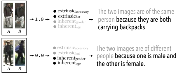
Figure 2. Explanations are constructed using cosine similarity on the predicted attribute probabilities. The model builds an explanation relative to its assessment of re-ID.
