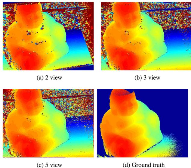
Figure 1. Comparison of depth estimated with different number of views are given: (a) 2 view, (b) 3 view, and (c) 5 view. In (d) ground truth, blue region represents non-depth values and background.
