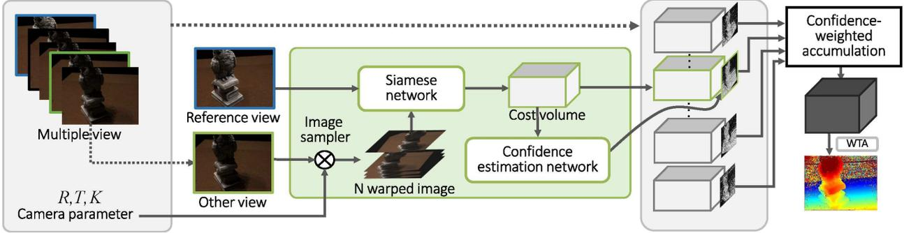
Figure 2. Overall architecture of generating cost volume in multi-view stereo. In order to train descriptors in multi-view stereo, descriptor network is proposed which consists of image sampler and siamese network. Also, for aggregating cost volumes generated by each two-views, we propose confidence estimation network. In multi-view stereo, the final matching cost in multiple view is made by confidence weighted sum of each cost volume.
