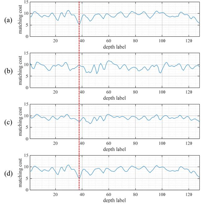
Figure 4. Explanation of effect of confidence weighting. (a) matching cost (correct), (b) matching cost (incorrect), (c) matching cost averaged, and (d) confidence weighted sum of matching cost. The red line shows the correct depth index.
