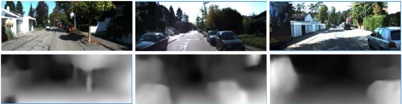
Figure 4: Qualitative results of depth prediction on KITTI dataset, where the network is trained in an unsupervised manner. Top row consists of target images and the bottom row consists of the corresponding predicted depth maps.
