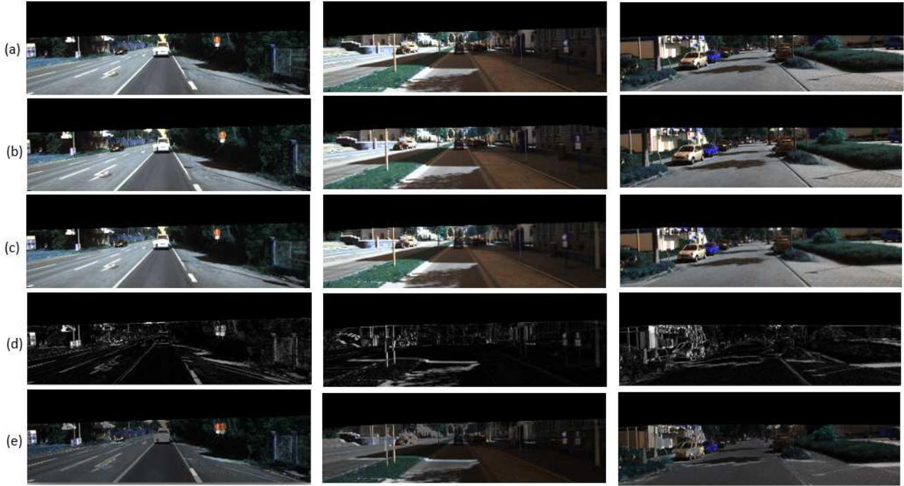
Figure 3: (a) Source images ( left ( I_{t-1} ) or right ( I_{t+1} )) (b) Target image (c) Generated (transformed source) image, using the estimated pose and depth parameters (d) photoconsistency error between generated (c) and (b), (e) Adversarial example with induced photoconsistency loss. The discriminator is trained with images in (a) and (b) as real vs. images (e) as fake. Image (e) has been enhanced with higher values of \omega ( =0.6 ) to amplify the difference for visual demonstration, but during training, the induced photoconsistency loss is kept lower.
