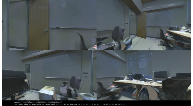
Figure 2: Captured frame from the evaluation environment. The four panes are different cameras in the scene, enabling multiple simultaneous viewpoints from the same agent. The bar at the bottom of the screen prints ground truth values that can easily be parsed by an OCR system.
