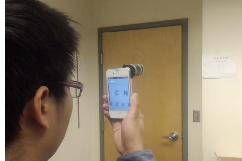
Figure 2: The stabilization app running on an iPhone 4S with an 6x optical telescope attached. The distant text on the wall is magnified and stabilized for ease of reading.
