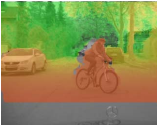
Figure 3: The SGM disparity map computed on the prototyping system. red=near, green=far.
