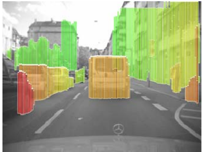
Figure 4: Based on Stixel representation, it is much less computation effort to analyze the scene.
