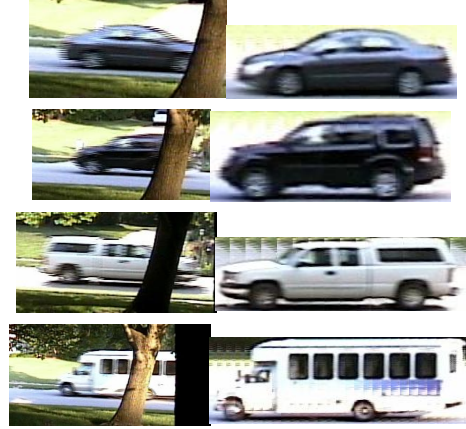
Figure 2. Sample four types of vehicles: sedan, van, pickup truck and bus are shown from top to bottom. Original image shots and their reconstructed results are shown on the left and right columns, respectively.
