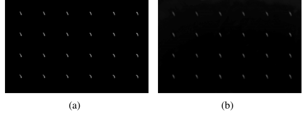
Figure 7. Testing on PSF accuracy using a point grid pattern. (a) synthetic result according to projective geometry. (b) blurred point grid pattern by our prototype optical computing system.
