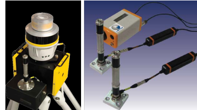
Figure 2. An iGPS transmitter and two sensor receiver bars (with cables and position computation engine).
