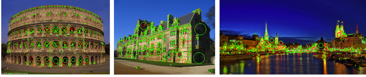
Figure 7: Blob detection using DoG implemented by VLFeat (green circles) and CABOX (red circles). Of those features detected with CABOX, 89 % are also detected by VLFeat while the remaining 11 % correspond to new features.
