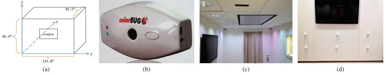
Figure 1: The testbed setup. (a) The coordinate system of the room. (b) The Seachanger wireless Colorbug sensor. (c) Twelve color controllable LED fixtures illuminate the room from the ceiling. (d) Color sensors are placed on the walls.
