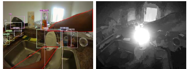
Figure 4. Experimental results of object detection and visual attention map: The left figure indicates that Step 3.1 provides individual objects and their regions. The right figure is generated in Step 3.2. It suggests that the user focuses strong attention on the central kettle.
