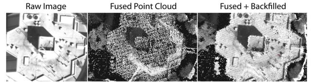
Figure 7: The left most figure shows the image of a top of a building from the CSUAV data set of Columbus Ohio (same building seen in figure 6). The middle image shows the image fused to the raw point cloud. The image on the right shows the image fused in a backfilled point cloud. The colors in the fused only point cloud are correct, but it can be hard to make out features given its sparseness. The back filled cloud is much easier to interpret and appears to be generally correct.
