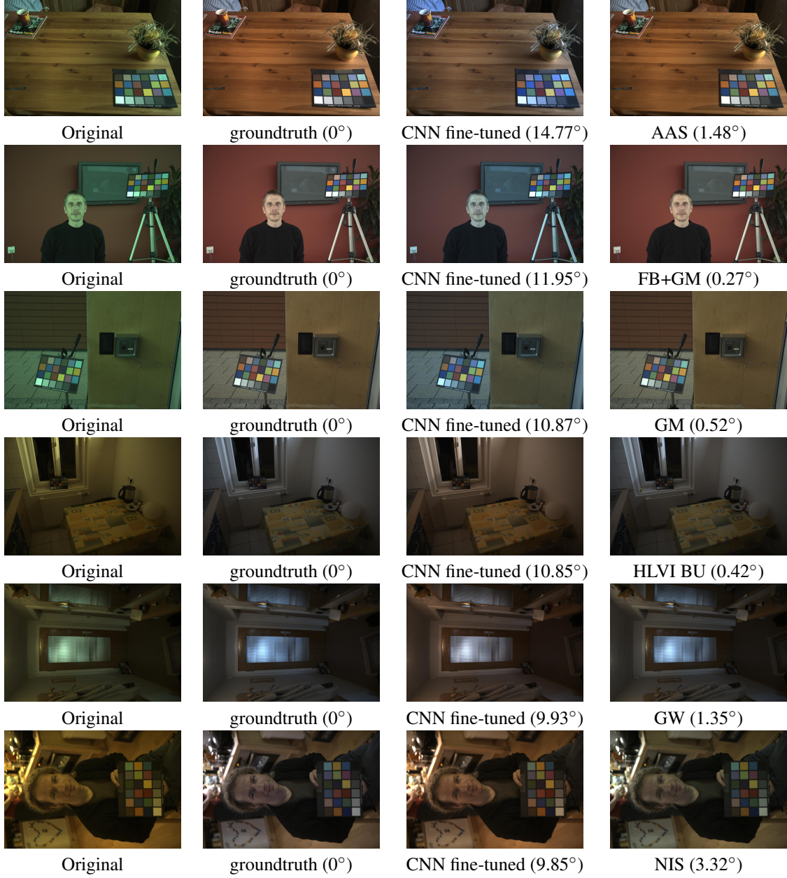
Figure 3. Examples of images on which the fine-tuned CNN makes the largest estimation errors. Left to right: original RAW image, correction with the groundtruth illuminant, correction with the CNN estimate, and correction with the algorithm in the state-of-the-art making the best estimate on the given image.
