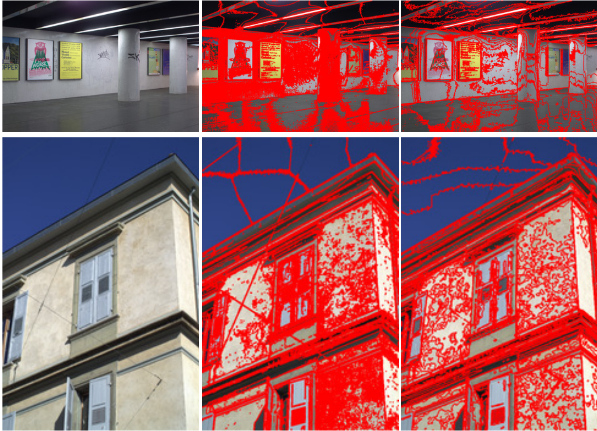
Figure 10. An example of the length metric. The top row is from the indoor category while the bottom row is from the urban category. The first column shows the original image, the second column shows the standard SLIC algorithm, and the third column shows the ISLIC algorithm.
