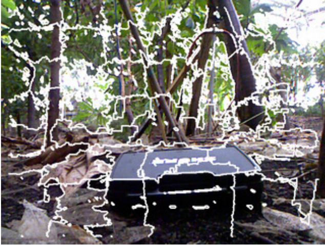
Figure 2. An example of how SLIC is sensitive to lighting conditions in unstructured environments. Note that the superpixels do not adhere to the bottom of the black box, nor to the leaves in the foreground.
