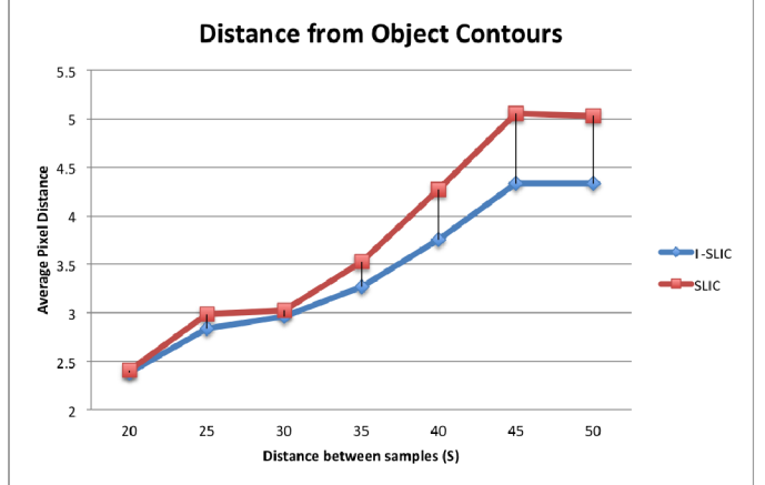
Figure 7. Comparing SLIC and ISLIC, varying the size of the superpixel. The graph shows the distance from the superpixel contour to the object contour.
