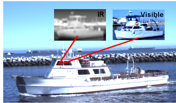
Figure 1. An example autonomous ship recognizing another vessel observed by both its IR and visible cameras. To follow international maritime traffic regulations, ASVs need to classify other ships during the day and in low-light conditions.
