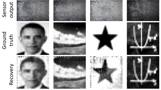
Figure 9. SparkleVision using board covered in glitter. Qualitatively the recovery is fairly close to the ground-truth light and a human can easily recognize the objects in the recovered image.
