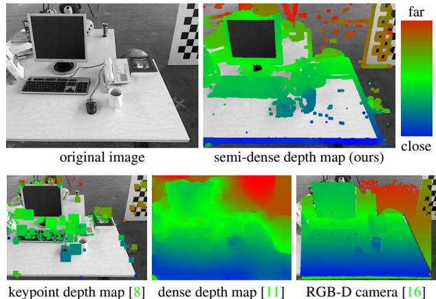
**Figure 2. Semi-Dense Approach:** Our approach reconstructs and tracks on a *semi-dense inverse depth map*, which is dense in all image regions carrying information (top-right). For comparison, the bottom row shows the respective result from a keypoint-based approach, a fully dense approach and the ground truth from an RGB-D camera.
