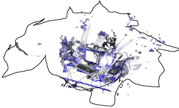
**Figure 9. RGB-D Benchmark Sequence fr2/desk:** Tracked camera trajectory (black), the depth map of the first frame (blue), and the estimated depth map (gray-scale) after a complete loop around the table. Note how well certain details such as the keyboard and the monitor align.
