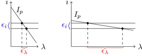
**Figure 6. Photometric Disparity Error:** Noise  $\epsilon_i$  on the image intensity values causes a small disparity error  $\epsilon_\lambda$  if the image gradient along the epipolar line is large (left). If the gradient is small, the disparity error is magnified (right).
