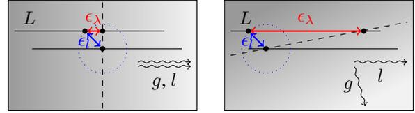
**Figure 5. Geometric Disparity Error:** Influence of a small positioning error  $\epsilon_l$  of the epipolar line on the disparity error  $\epsilon_\lambda$ . The dashed line represents the isocurve on which the matching point has to lie.  $\epsilon_\lambda$  is small if the epipolar line is parallel to the image gradient (left), and a large one otherwise (right).
