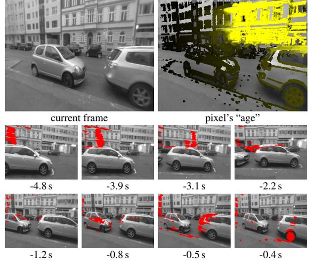
**Figure 4. Adaptive Baseline Selection:** For each pixel in the new frame (top left), a different stereo-reference frame is selected, based on how long the pixel was visible (top right: the more yellow, the older the pixel.). Some of the reference frames are displayed below, the red regions were used for stereo comparisons.
