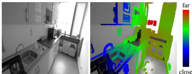
**Figure 1. Semi-Dense Monocular Visual Odometry:** Our approach works on a semi-dense inverse depth map and combines the accuracy and robustness of dense visual SLAM methods with the efficiency of feature-based techniques. Left: video frame, Right: color-coded semi-dense depth map, which consists of depth estimates in all image regions with sufficient structure.
