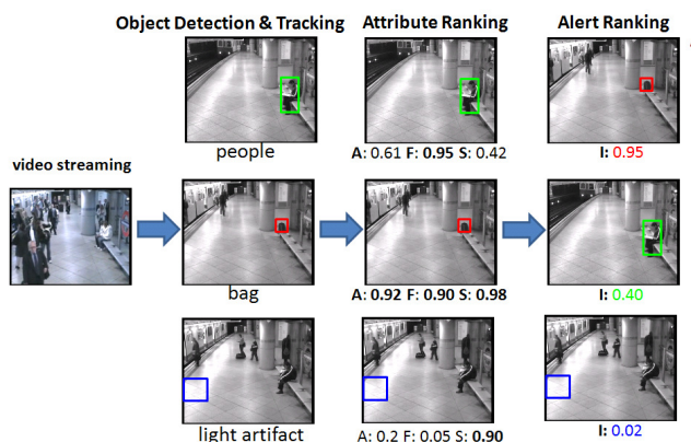
Figure 1: An overview flow chart of our system (best view in color). An abandoned object tends to indicate high staticness (S), foregroundness (F) and abandonment (A). Our approach applies the technique [19] to learn the strengths of these visual attributes (shown below each image). These high-level attributes are then fed to a second level ranker to prioritize the importance (I) of an object. Alerts are sorted (3 rd column) by importance and finally triggered if their relevance scores are high. (image courtesy of iLIDS [2])
