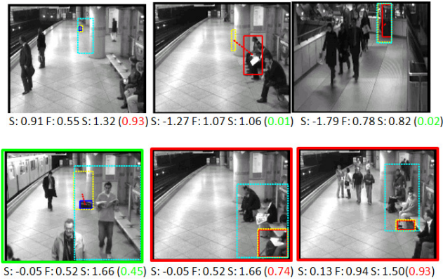
Figure 7: Example alerts provided by our system. The top row shows correct detections while the bottom row illustrates false detections (a false positive is highlighted with a red bounding box around the image while a green box indicates a false negative). Shown in the brackets are the ranking scores of the alerts. Also see Fig. 4 for explanation of the bounding boxes.
