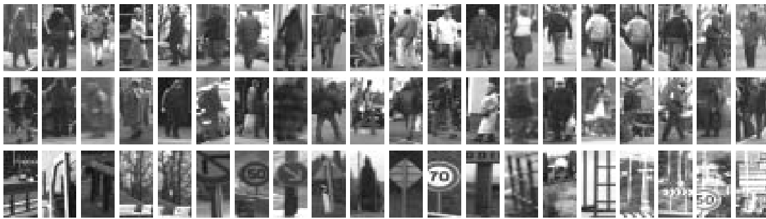
Figure 7. Some samples of (top) true detection of pedestrian (true positive), (middle) false detection of non-pedestrian (false negative), and (bottom) false detection of pedestrian (false positive).
