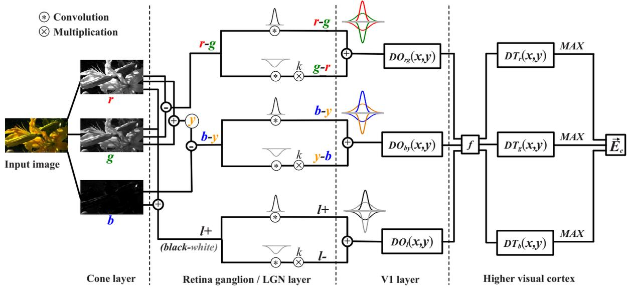
Figure 3. The flowchart of our double-opponency based color constancy model. The symbol  $f$  indicates the linear transform defined by Equation (5).  $r$ ,  $g$ ,  $b$ ,  $y$ , and  $l$  denote respectively the components of the red, green, blue, yellow and luminance channels.  $MAX$  denotes the mechanism of MAX.
