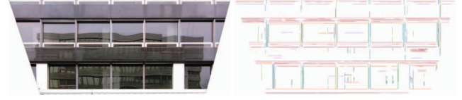
Figure 3. Ortho-rectified input image (left) and oriented edge image (right): Vertical edges are in green and blue (positive and negative gradient), horizontal ones are in red and magenta.
