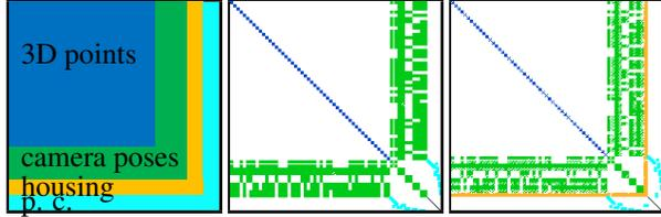
Figure 4. Sparse matrices for refractive bundle adjustment. Left: general block structure of sparse matrix  $N$ . Middle: optimization of 3D points and camera poses. Note that only colored parts are non-zero. Right: additional optimization of housing parameters. Colors: 3D points blue, poses green, housing parameters orange, constraints between parameters cyan.
